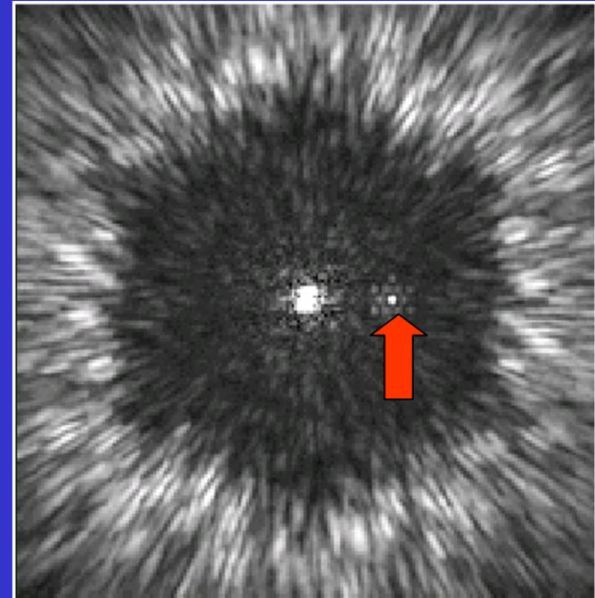
*Simulated NGST coronagraphic image of a planet around Lalande 21185 (M2V at 2.5 pc) at 4.6  $\mu$ m*
