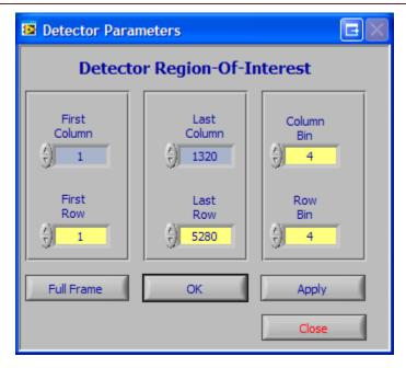
Pressing the Detector button opens the Detector Parameters window shown above. The row and column numbers are always specified in unbinned pixels. The binning may also be changed on the main window directly.
