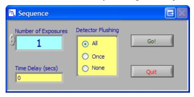
The Sequence button opens the Sequence window above which makes a series of exposures, all of the same ImageType. For a sequence, auto increment sequence in Image Filename should usually be turned on to increment the image sequence number by one after each exposure. For Comparison exposures, opening the Sequence window turns on the selected comp lamp and closing the window turns off the same lamp.
