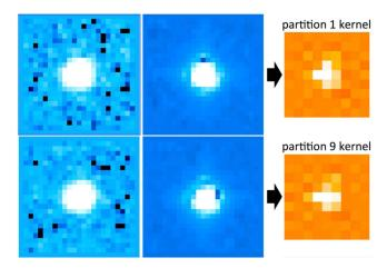
**Figure 7.** Example PSF image products for two separate image partitions: top row corresponds to a partition at the bottom left of a CCD image and bottom row is for a partition at top right of the same image. From left to right: PSF for science image, PSF for reference image, and the resulting PSF matching kernel derived using the method in Section 4.7. Pixel sizes are the same throughout. The kernel images are enlarged for clarity.
