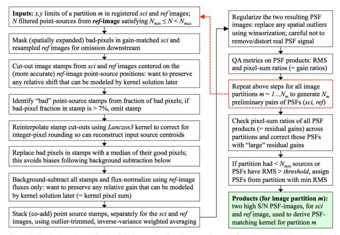
**Figure 6.** Processing flow for the creation and allocation of PSF image products for each common science and reference image partition. These are used to derive the spatially dependent PSF-matching kernel between the science and reference image. See Section 4.6 for details.
