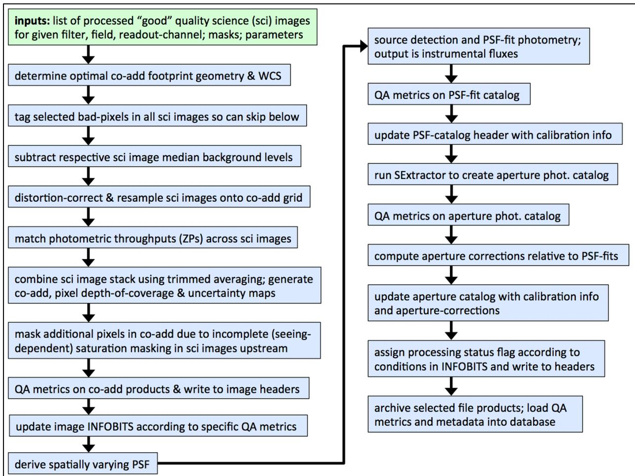
**Figure 11: High-level processing flow in the reference image (co-add) generation pipeline. For details, see Section 6.7.**
