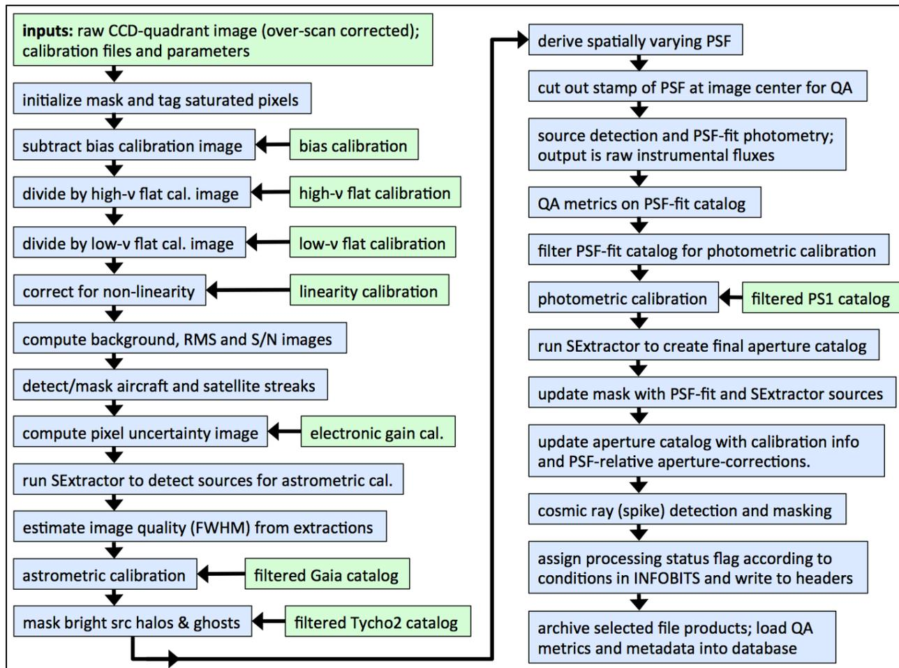
**Figure 4: High-level processing flow in the instrumental calibration pipeline. This represents the first phase of the real-time pipeline. For details, see Section 6.5.**
