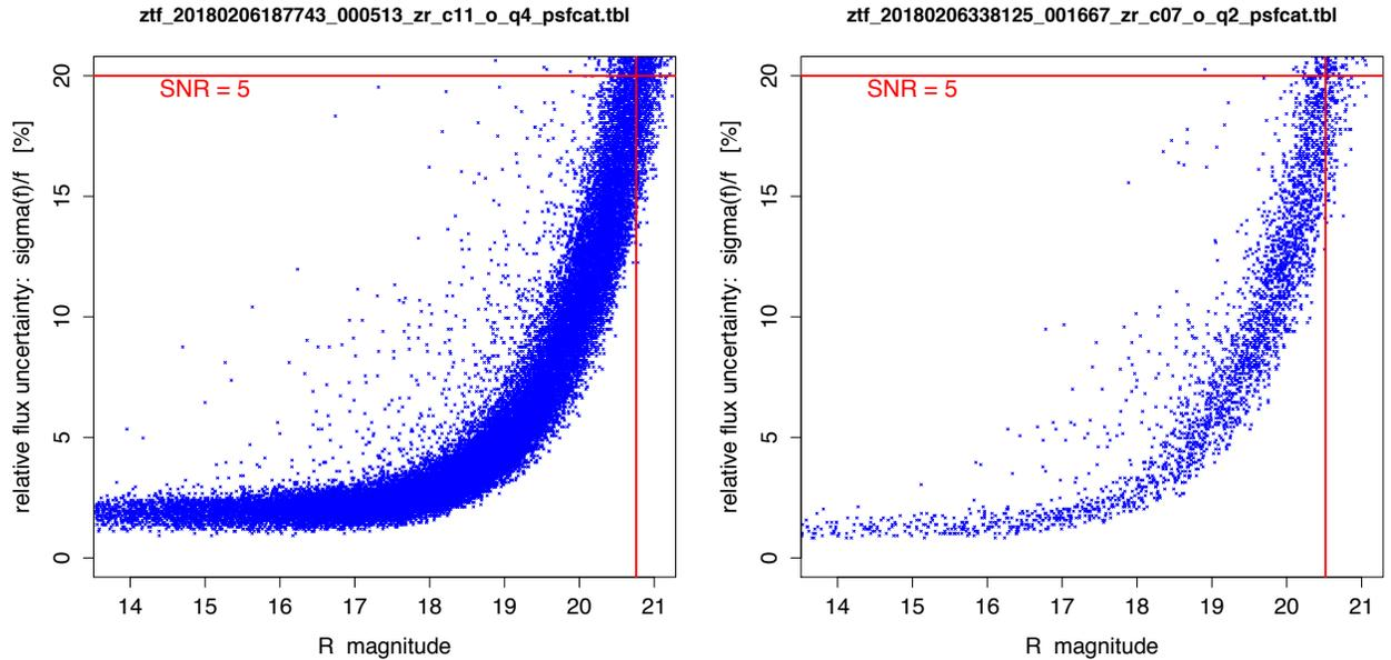
**Figure 22: relative (model-based) flux uncertainty as reported in two PSF-fit catalogs, for a dense galactic plane field (*left*) and a high galactic latitude field (*right*). Vertical lines correspond to the approximate 5- $\sigma$  magnitude limits (20% flux-uncertainty cut).**
