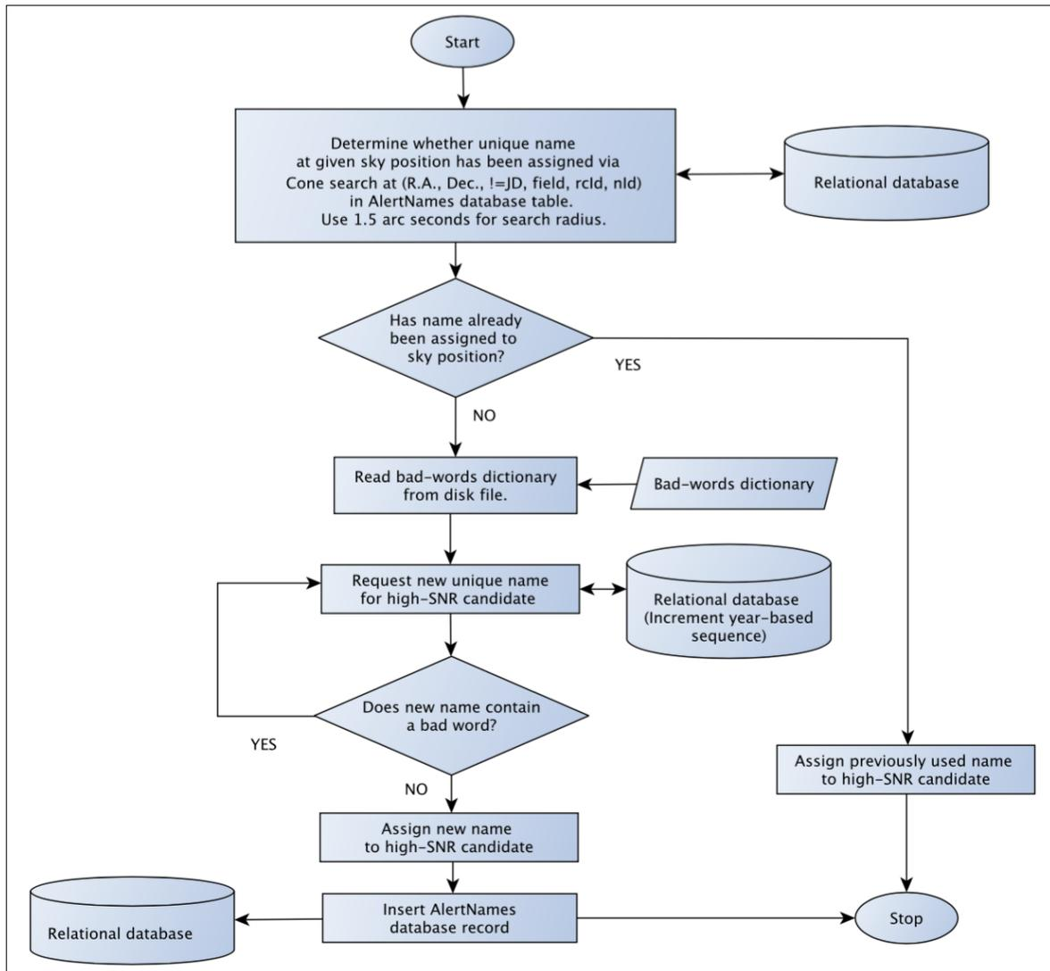
Figure 13: Process used to assign or re-assign names (*objectId*) to alert packets
