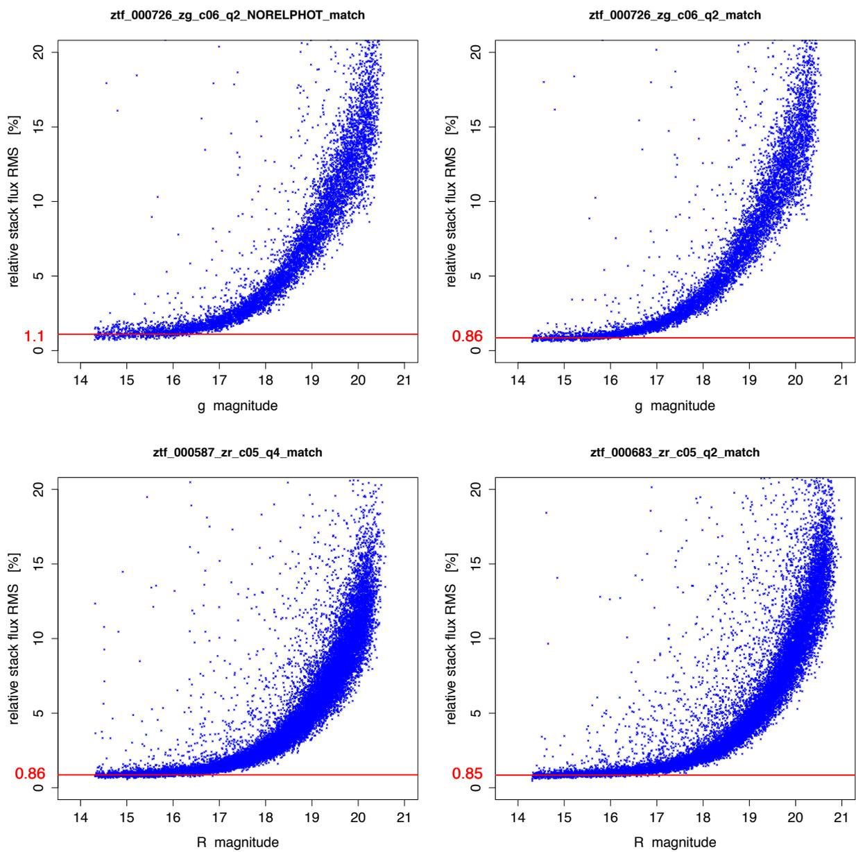
**Figure 19: Relative flux RMS in stacked multi-epochal photometry (repeatability) extracted from *matchfile* products. The inputs are PSF-fit catalogs. The *top left and right panels* correspond to the same field/readout-quadrant image and are for runs where the relative-photometric refinement step was turned off and on respectively.**
