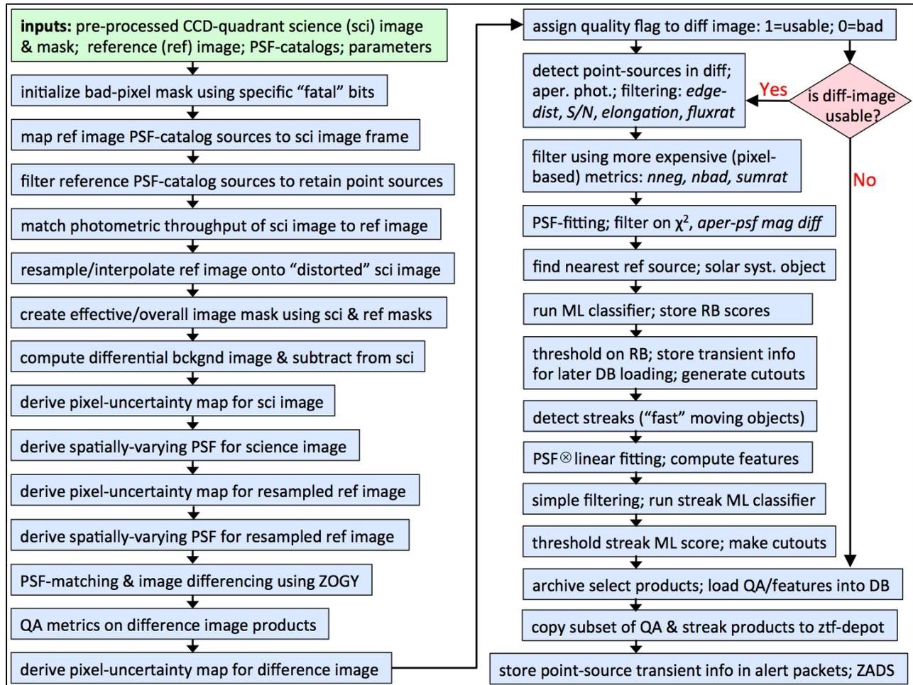
**Figure 10: High-level processing flow in the image-subtraction and transient (point-source and streak) extraction pipeline. This represents the second phase of the real-time pipeline (the first was shown in Figure 4). For details, see Section 6.6.**
