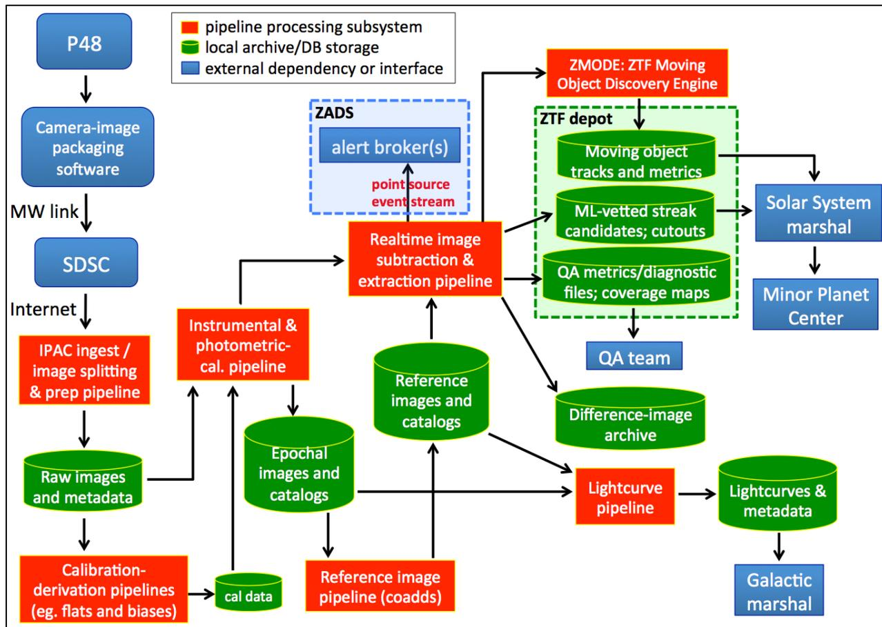
Figure 2: Pipeline-level data flow in the ZSDS. **Green** components indicate storage in the form of an archive and/or database residing at IPAC to serve either the public, science marshals (via ZTF-depot) or the collaboration. Specific products are summarized in Section 7. **Red** components represent the core pipelines. Further details on the pipelines are given in Section 6. **Blue** components indicate external interfaces or dependencies.
