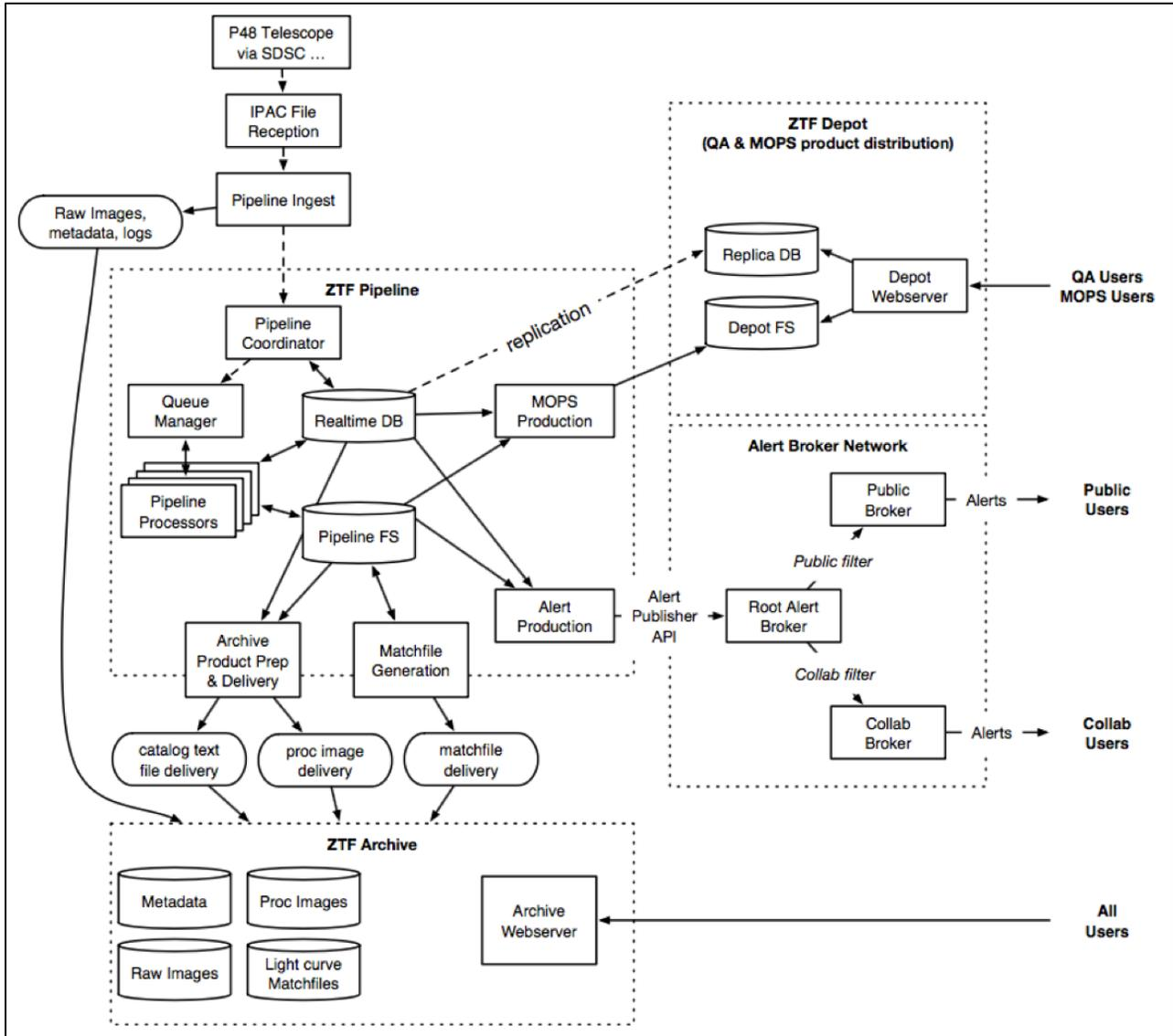
**Figure 3: High-level design of the ZSDS, showing databases, file systems, and interfaces. The “ZTF Pipeline” and “ZTF Depot” boxes are expanded in Figure 2.**
