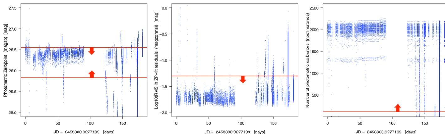
**Figure 27: trends in  $magzp$ ,  $magzprms$ , and  $nps1matches$  per CCD quadrant in  $r$ -filter exposures for survey field 806 from 2018-07-01 to 2018-12-29. Red lines with arrows indicate approximate thresholds for “good” (usable) image data. Data outside these limits are flagged in the archive metadata. See cautionary note (2) in Section 3.4.**
