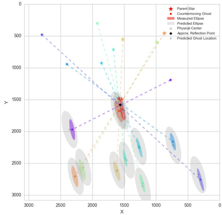
**Figure B2: Schematic showing locations of parent stars and their counter-moving ghosts. The ghosts shown here *will not* actually appear in the same CCD quadrant as their parents. They would be masked in *another* quadrant reflected through the FOV center (optical axis).**
