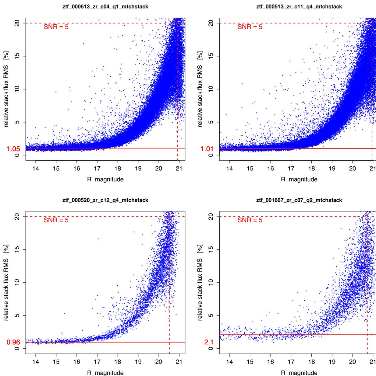
**Figure 20: Independent estimates of the relative flux-RMS in stacked multi-epochal photometry (repeatability) using the PSF-fit catalogs. Unlike Figure 19, these do not use the *matchfile* products, but are based on matching the catalogs directly. Vertical dashed lines correspond to the approximate 5- $\sigma$  magnitude limits (20% flux-RMS). See Section 12.2 for details.**
