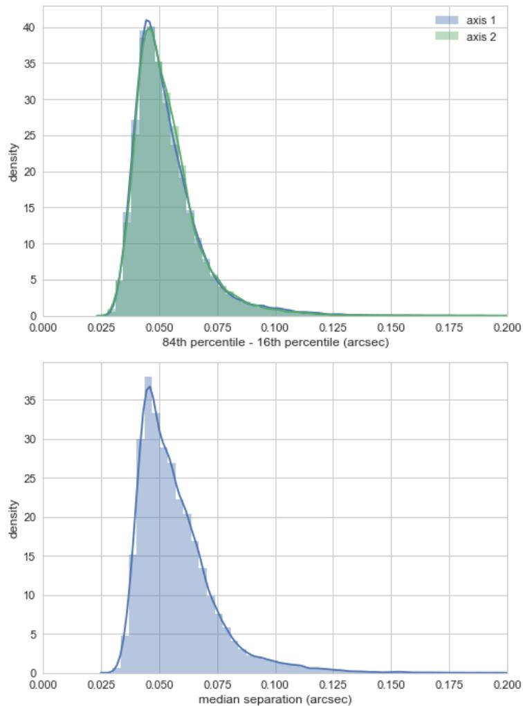
**Figure 17: overall astrometric accuracy per processed quadrant image with respect to *Gaia* DR1. Top: distribution in robust estimate for the RMS deviation based on half the 84<sup>th</sup> - 16<sup>th</sup> percentile range where axes 1,2 = R.A., Dec. Bottom: distribution in the median radial separation.**
