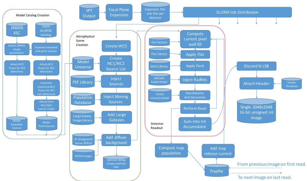
Figure 1 - architecture of the NEO Surveyor image simulator
